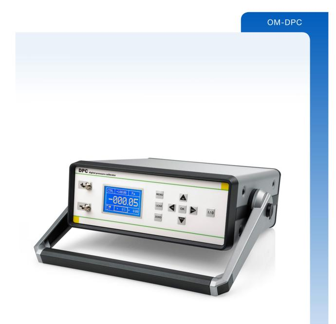
The OM-DPC measures and generates pressures and consequently it is more than a mere measuring instrument – it can also be applied as test and calibration instrument for pressure sensors and pressure switches. Thanks to internal pressure generation no auxiliary tools are required for operation. An internal Li-ion battery is available for mobile operation. Parallel operation of mains and battery supply allows for maximum flexibility.
