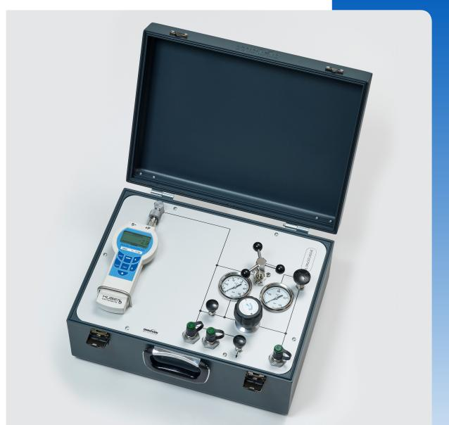
The portable calibrator OM.H-DM 591/592 is used to make pneumatic tests and calibrations of measurement and control equipment during commissioning and inspections. The high-pressure calibrator is suitable for simulating overpressure. Air or nitrogen pressures up to 90 bar can be simulated, depending on the equipment. A compressed air or nitrogen bottle with a capacity of 2 litres and a nominal pressure of 200 bar is integrated in the calibrator, and can be filled through a filler neck.
